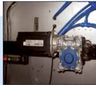
Servo drive with integrated breaking facility for paper pull for precise control of pouch height.
